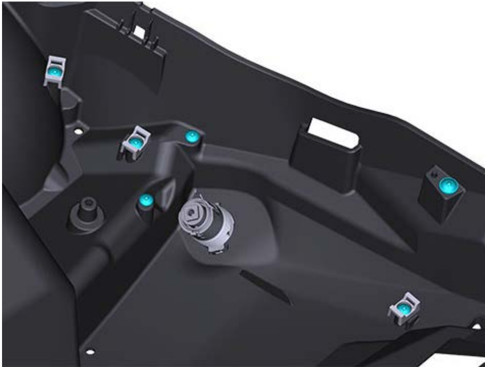
Fit plate (26) by engaging lock tabs (A) and (B) in the recesses.
