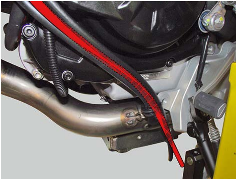
Positioning the fuel pipes.
